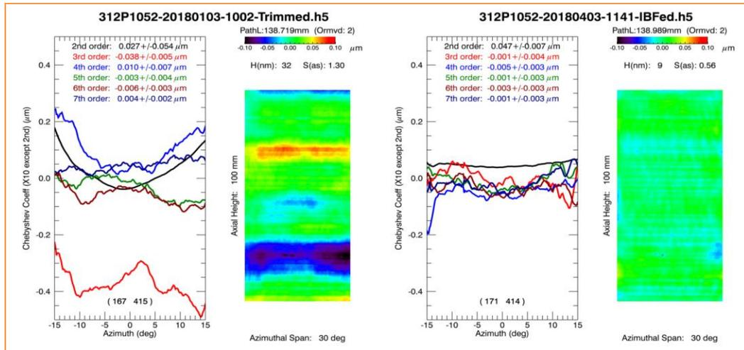
Fig. 8 Sample 312P1052 before and after the figuring
