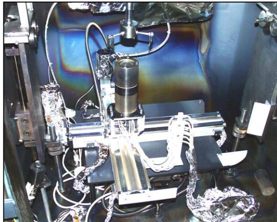
Fig.. 3 IBF facility for optics up to 300 mm
