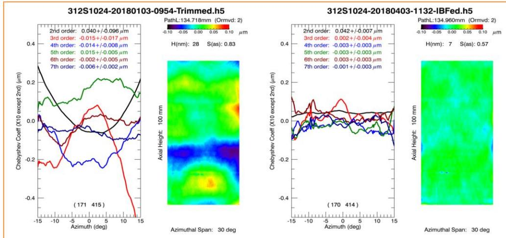
Fig. 11 Sample 312S1024 before and after the figuring
