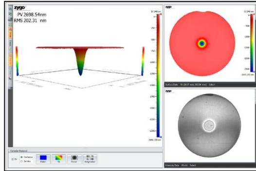
Fig. 1 Interferometric measure of the “hole” created on a 100 mm Silicon sample made to obtain the RF (10 min exposure)
