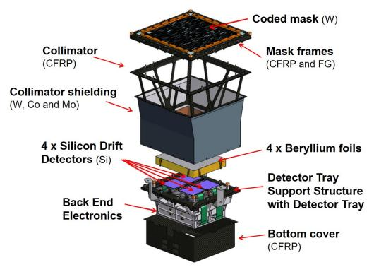
Figure 10. An exploded view of a STROBE-X/WFM camera, indicating all its components.
