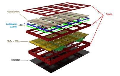
Figure 7. An exploded view of the STROBE-X/LAD module frame design, based on the design for the ESA LOFT mission concept.
