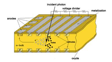
Figure 8. Working principle of the Si drift detector used for the STROBE-X/LAD (see text for details).
