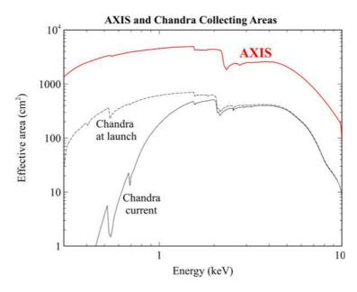
Figure 2. Comparison of the AXIS collecting area including detector efficiency and filters to that of Chandra at launch. The lower line shows the effect of the growth of contamination on the Chanda ACIS detector.
