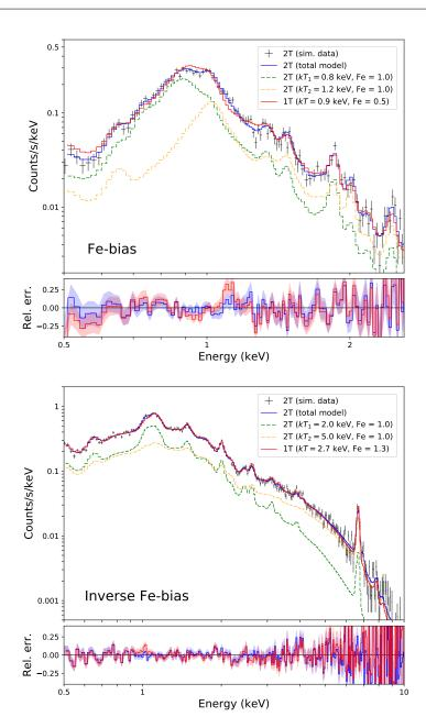
**Fig. 10** Illustration of the Fe-bias (top) and the inverse Fe-bias (bottom). In both bases, a two-temperature plasma (2T; with temperatures  $kT_1$  and  $kT_2$ ) is simulated through an EPIC MOS spectrum, which is then re-fitted using a single-temperature component (1T). In both cases, the 2T and 1T fits (blue and red lines, respectively) provide very similar spectra, yet with different Fe abundances.
