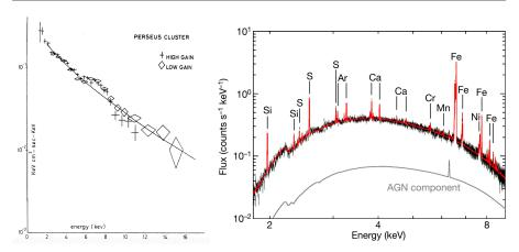
Fig. 2 Left (from Mitchell et al. 1976, reprinted with permission): X-ray spectrum of the Perseus cluster core seen by the MSSL collimated proportional counter onboard Ariel V. Right (from Hitomi Collaboration et al. 2017, reprinted with permission): X-ray spectrum of the Perseus cluster core seen by the SXS instrument onboard Hitomi.
