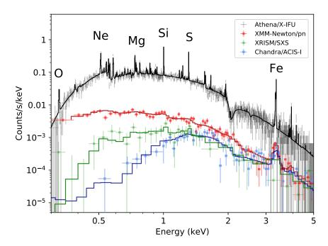
Fig. 11 Simulated 250 ks spectrum of the core of a distant cluster ( $kT=3~{\rm keV},\,z=1$ ) with the Athena X-IFU instrument. For comparison, similar simulated spectra are also shown for the XMM-Newton pn, Chandra ACIS-I, and Hitomi/XRISM SXS instruments. For clarity, the data points have been rebinned.
