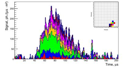
**Figure 3:** Light curve of the TUS161003 event as the sum of signals in the ten hit channels. The signal is smoothed with a moving average calculated for three time steps to minimize statistical fluctuations. The average background illumination was extracted. The inset shows positions of the hit pixels in the focal surface.
