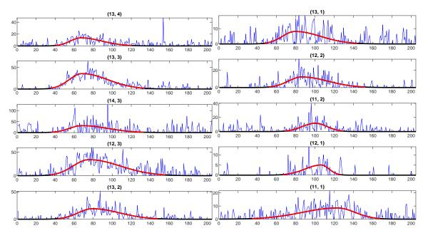
**Figure 2:** Signals in ten hit channels of the TUS161003 event with bi-Gaussian approximations. The average level of background illumination is extracted from the signals for clarity. Numbers in parenthesis above the panels indicate the module and channel numbers respectively. The *x*-axes represent time in  $\mu$ s.
