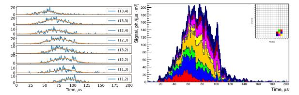
**Figure 4:** The TUS detector response to an EAS generated by a 1 ZeV proton arriving at  $\theta \approx 50^{\circ}$ . Left: ADC codes of eight hit channels. Right: the light curve. The inset shows positions of the hit pixels in the focal surface.
